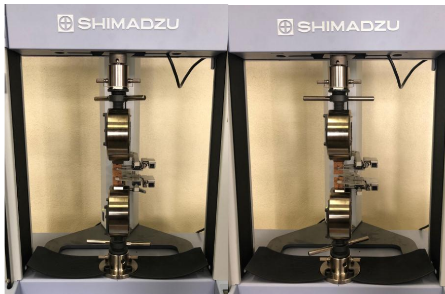
Figure 4 Shimadzu Autograph AGS-X series Europa testing machine used for the adhesive films and cork composites characterization.
