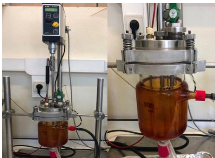
Figure 3 Reactor designed by the LSRE-LCM group for the synthesis of aqueous polyurethane dispersions.
