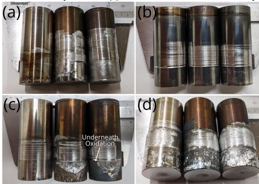
Figure 34 - Samples after aluminum ring extraction. From left to right: simple cast, 10 minutes and 30 minutes aluminum contact. (a) AISI H13, (b) AISI H13 coated with AlCrN PVD, (c) AISI H13 coated with H13 by HVOF and (d) AISI H13 coated with Cr 3 C 2 25NiCr by HVOF.
