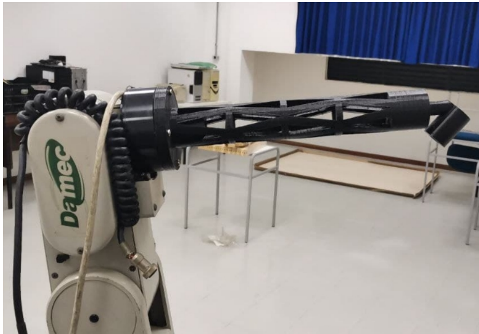
Figure 8 – Close-up view of the microphone holder.
