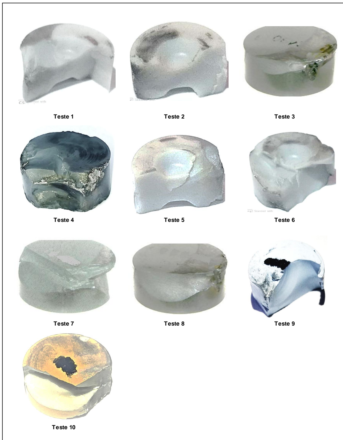
Figura 56 – Falha catastrófica nos insertos \text{Al}_2\text{O}_3 + \text{SiCw} e \text{Al}_2\text{O}_3 + \text{ZrO}_2
