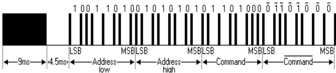
Figura 18 - Extended NEC Protocol
